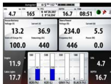
CZone integration - battery and tank monitoring
